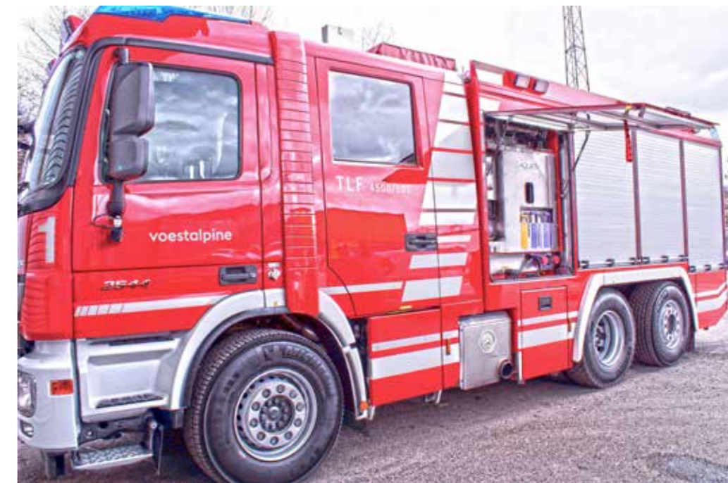
Fire vehicle with integrated high-pressure water mist unit to supply semi-stationary systems.
